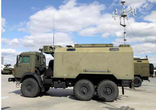
Vitaly Kuzmin A Russian R-330Zh Zhitel electronic warfare system, which is used to jam cellular satellite communications.
